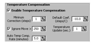
You should recognize most of the parameters as being the same as those on the **Control** panel on the **Temp Control** tab. The settings here allow you to set those values you wish to be inserted into the **Control** panel when FocusAide is started. There are two additional controls on this panel.
