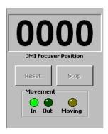
You should recognize this as the same status panel as presented on the Manual and Auto Focus tabs. The current focuser position is shown along with movement and direction indicators. The **Reset** and **Stop** buttons operate as usual on this page but are disabled if Automatic Compensation is in progress. Turning off automatic compensation will not stop any focuser movement in progress. Use the **Stop** button on this panel to do so if desired.
